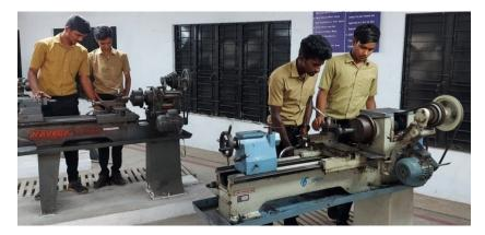
This lab consists of Centre Lathe & All geared Lathe and the function of lathe machines are Turning, Facing, Knurling, Tapering, Grooving and Threading etc.
