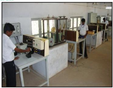
This lab has facilities like Generators, Induction motors power supply, ammeter, voltmeter, wattmeter and Rectifier.
