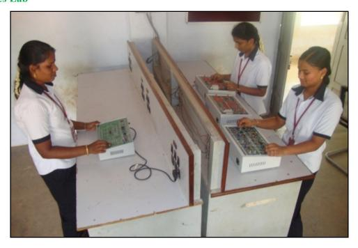
The Lab focuses on Electronic Devices and Circuits, Electrical Circuits and Instrumentation experiments, Analog and Digital Experiments and Industrial Electronics experiments. The Lab has power supplies of various ranges, function generators and Cathode Ray Oscilloscopes.
